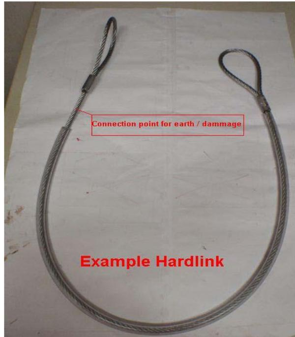
Figure 1 - Typical metal 'hard-link' for rope access technicians
