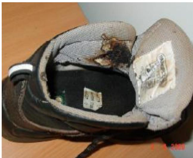
Figure 2 – Injured person's safety shoe showing burn damage
